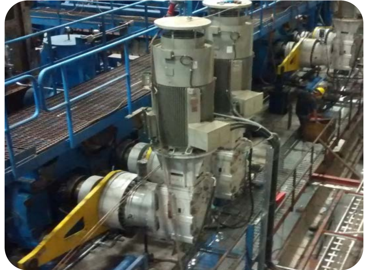
Fig: Actual installation at San Diego, Gautemala Site having Top Roller with Foot mounted drive and Bottom Rollers with Shaft mounted drive
