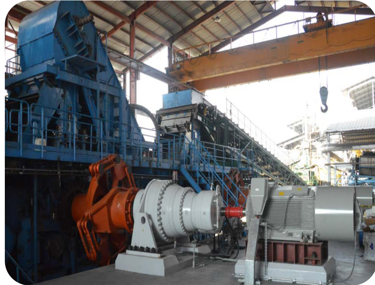
Fig: Actual installation at San Diego, Gautemala Site having Top Roller with Foot mounted drive and Bottom Rollers with Shaft mounted drive
