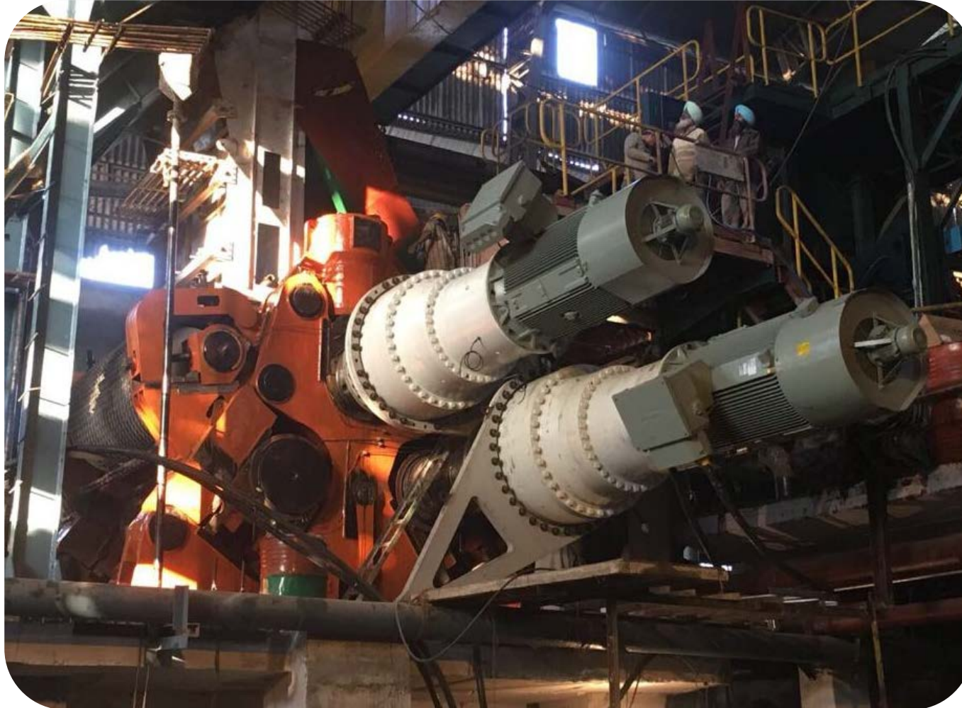
Fig : In Line Shaft mounted drive on Top, feed & discharge roller – ISL, Mukerian, Punjab
